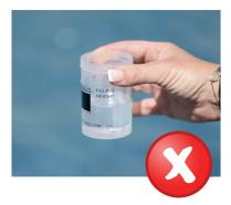
Use the measuring cup provided and make sure that the water level is correct. Here, the cup is not filled sufficiently. This means that the LILIAN cannot pump the water sample correctly into the SensoStick, resulting in an error message.
