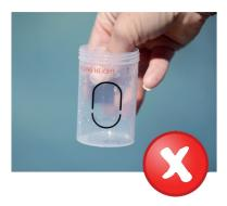
Please do not touch the sample cup! Residues of your fingerprint cause the free chlorine in the water sample to react with the combined chlorine. This falsifies the measurement result.
