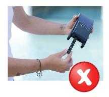
In this example, the SensoStick is inserted from the wrong direction.
