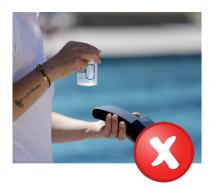
It should never be measured without the measuring holder, because the LILIAN must be in a vertical position during the whole measurement.
