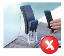
The flap of the handheld meter must be closed for each measurement. This minimizes the influence of stray light.
