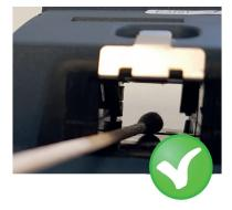
The easiest way to clean the measuring channels is with a cotton pad moistened with isopropanol. During cleaning, perform gentle, circular movements in the measuring slot.
