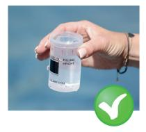
The cup should be filled with the water sample up to the thread.
