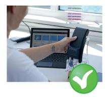
Here the LILIAN is placed in the special measuring holder. This has suitable recess and ensures that the LILIAN cannot change position during the measurement.
