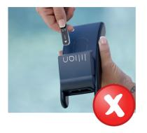
The part of the stick that is in the water sample must not be touched. The free chlorine of the water sample will otherwise react with traces of the fingerprint on the SensoStick and you will measure increased combined chlorine values.
