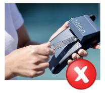
The SensoStick must not be inserted with the printed side down.
