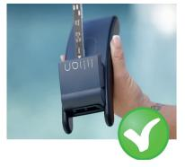
The stick is only ever touched at the back when it is inserted into the measuring device in order to prevent deviations in the measurement result.
