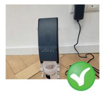
Here the measurement can take place because the charger is not plugged in. A minimum charge level of 10% is required to perform a measurement.
