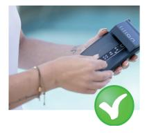
The SensoStick is always inserted into one of the two slots with the printed side facing up.
