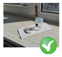
We recommend storing the cups open and with the open side facing down, e.g. on kitchen roll, until they are dry. If you want to wipe the cups dry with a cloth, please take care not to get any particles or impurities into the cup. Replace the measuring cups after one month of use at the latest.
