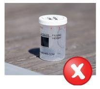
The measuring cup must be sufficiently rinsed and cleaned before and after each measurement. Do not store the wet cups with the lid closed. This can cause germs to form, which can lead to an incorrect chlorine value at the next measurement.
