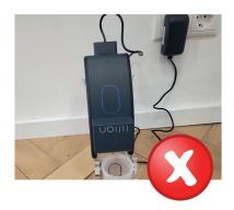
For safety reasons, the device cannot be charged during a measurement. Therefore, remove the charging plug during the measurement.
