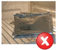
The storage temperature for the SensoSticks is 0-30 °C. However, we do not recommend storing them in the refrigerator, as they must first warm up to room temperature before they can be used. Otherwise, the SensoSticks will mist up and the measurement may be falsified.
