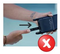
The SensoStick is always pulled out of the slots of the LILIAN device from the back to the front.
