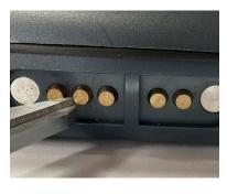
If this does not help either, you must reset the LILIAN measuring device completely. To do this, bridge the two outer PINs of the 3-PIN combination on the device with a conductive object such as a paper clip, scissors or the springs from the maintenance kit. After approx. 1 second, the device vibrates and the reset is successful.
