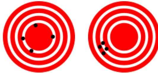
In the left figure, the hits show high accuracy but low precision: the readings fluctuate widely around the correct value. In the figure on the right, the accuracy is low but the precision is high: The measured values hardly fluctuate but around the wrong value (image source: Wikipedia).
