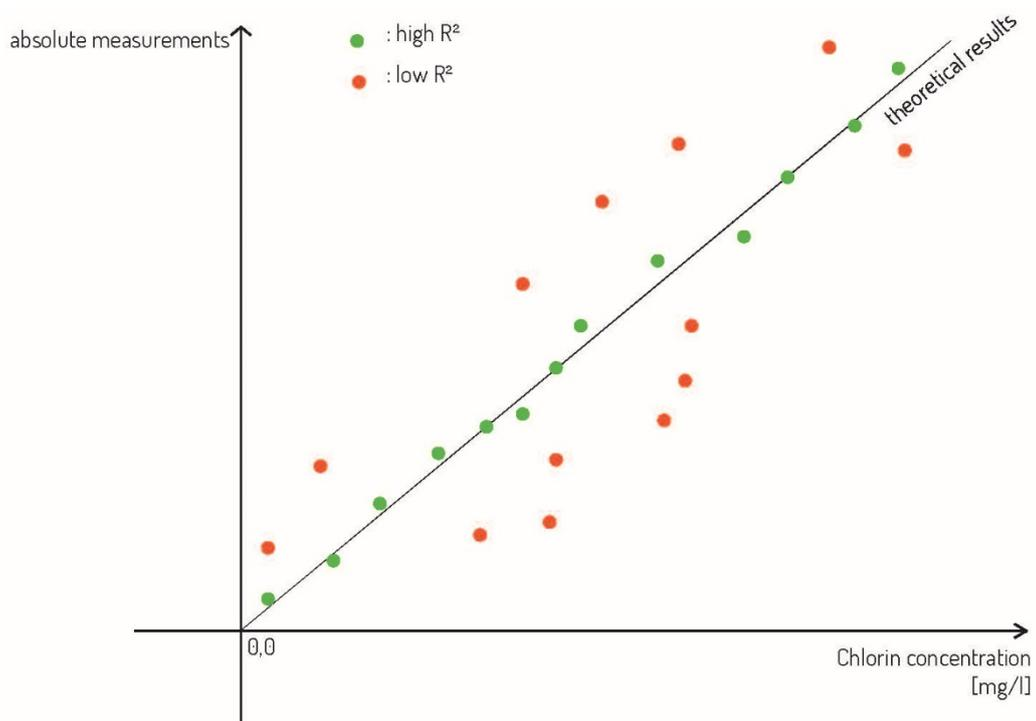
The different colours of the measured values (red and green) represent two measurement series. The theoretical target values are drawn as a line. The following applies: The closer the measured values are to the line, the higher the accuracy (not only the precision) of the measuring device.
