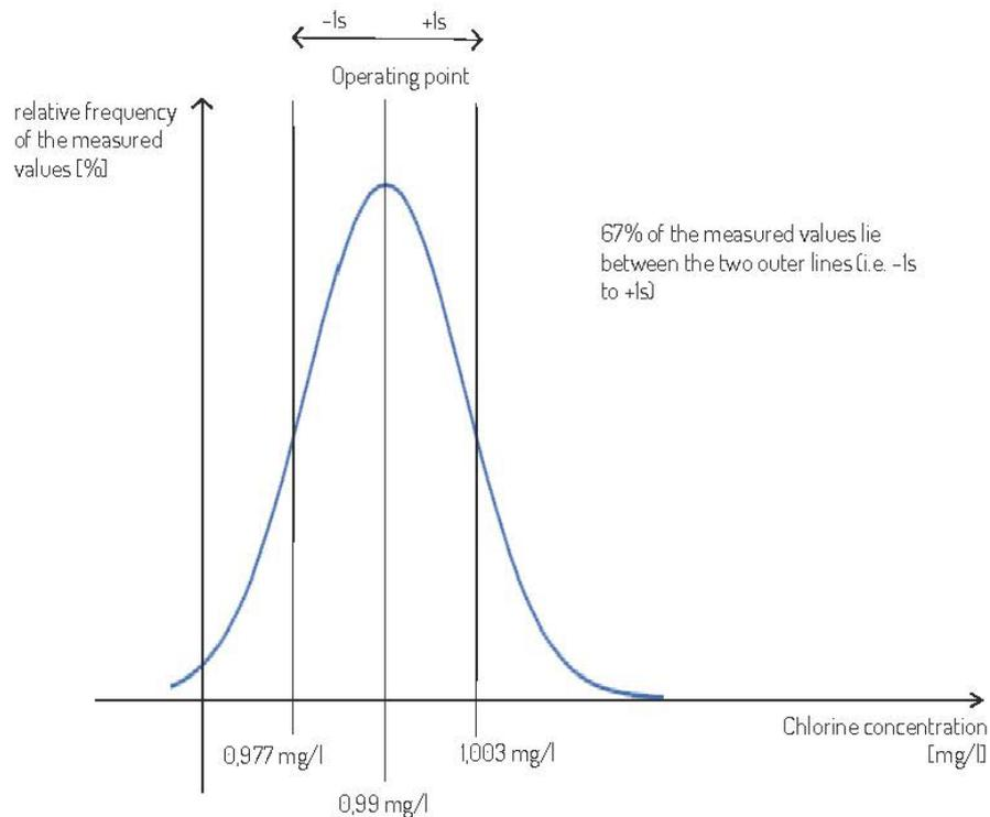
Here a problem becomes apparent: If a measuring device achieves this precision in only 2 out of 3 cases, the statement for a practical application is rather low. Therefore, the confidence range was still given at 1.00 mg/l free chlorine ( $\pm 0.021$  mg/l): In 95 out of 100 measurements, the measured values ranged from 0.979 mg/l to 1.021 mg/l. The operating point for this is 1.00 mg/l free chlorine, as this is a typical working value for swimming pool applications.
