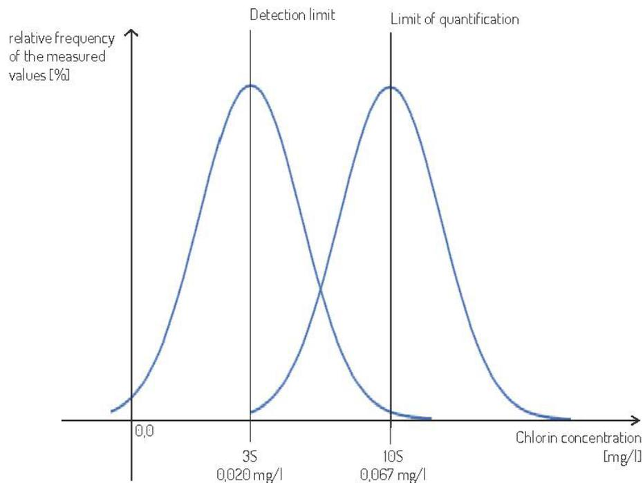
Drawn in blue are the possible measurement results of the meter with their relative frequency at different chlorine concentrations. This is called a measured value distribution. It is gaussian, i.e. the middle measured value is most likely to be measured and the probability of measuring corresponding values decreases towards higher and lower measured values up to 0% probability.
