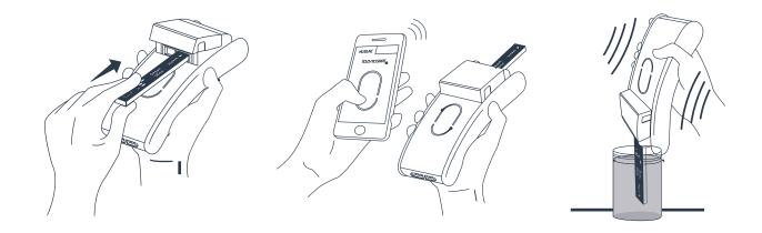
Simply insert the SensoStick into the LILIAN, connect it to the app and start the measurement at the touch of a button. The rest of the measurement process takes less than a minute. The measuring accuracy complies with DIN19643.
